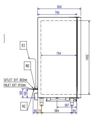
Drain Electrical inlet (power) RO Refrigerant Outlet
